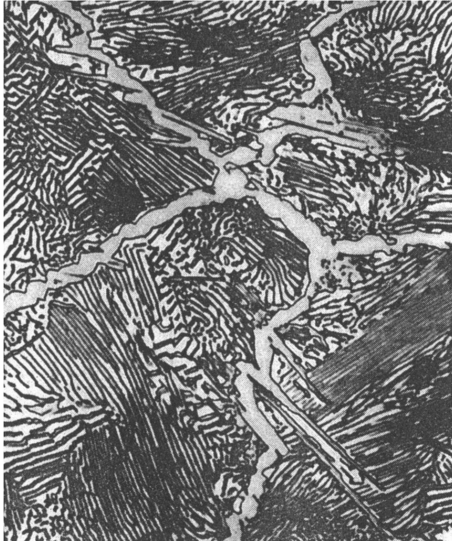
Figure 9.31 Photomicrograph of a 1.4wt% C steel having a microstructure consisting of a white proeutectoid cementite network surrounding the pearlite colonies. 1000 \times . (Copyright 1971 by United States Steel Corporation.)
