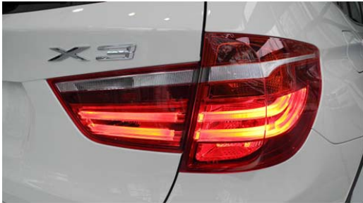
Fig. 1. Example of automotive tail lamp using LED end-lit light guide bars [2]
