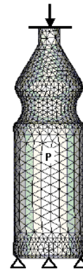
Fig. 9 The mechanical loading of the blown bottle: internal pressurization and top displacement.
