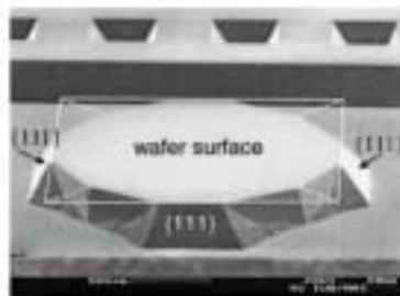
Fig. 1. Scanning electron micrograph (SEM) of an anisotropically etched \text{Si}(100) micro structure showing UC undercutting. The shape of the square etchback is indicated (0.33 \mu\text{m}^2 100\text{nm} \times 100\text{nm} ).
