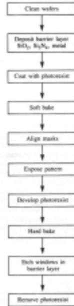
Fig. 2.1 Steps of the photolithographic process.
