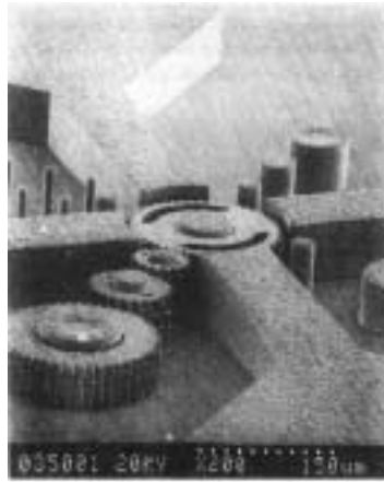
圖 4.33 使用 LIGA 技術的微馬達 - 感謝 the University of Wisconsin-Madison (Department of Electrical and Computer Science)
