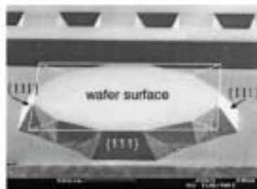
Fig. 1 Scanning electron micrograph (SEM) of an anisotropically etched Si (100) micro structure showing UC undercutting. The shape of the rounded sidewall is indicated (0.33 μm 2 x2000x/0.5 μm 2 ).
